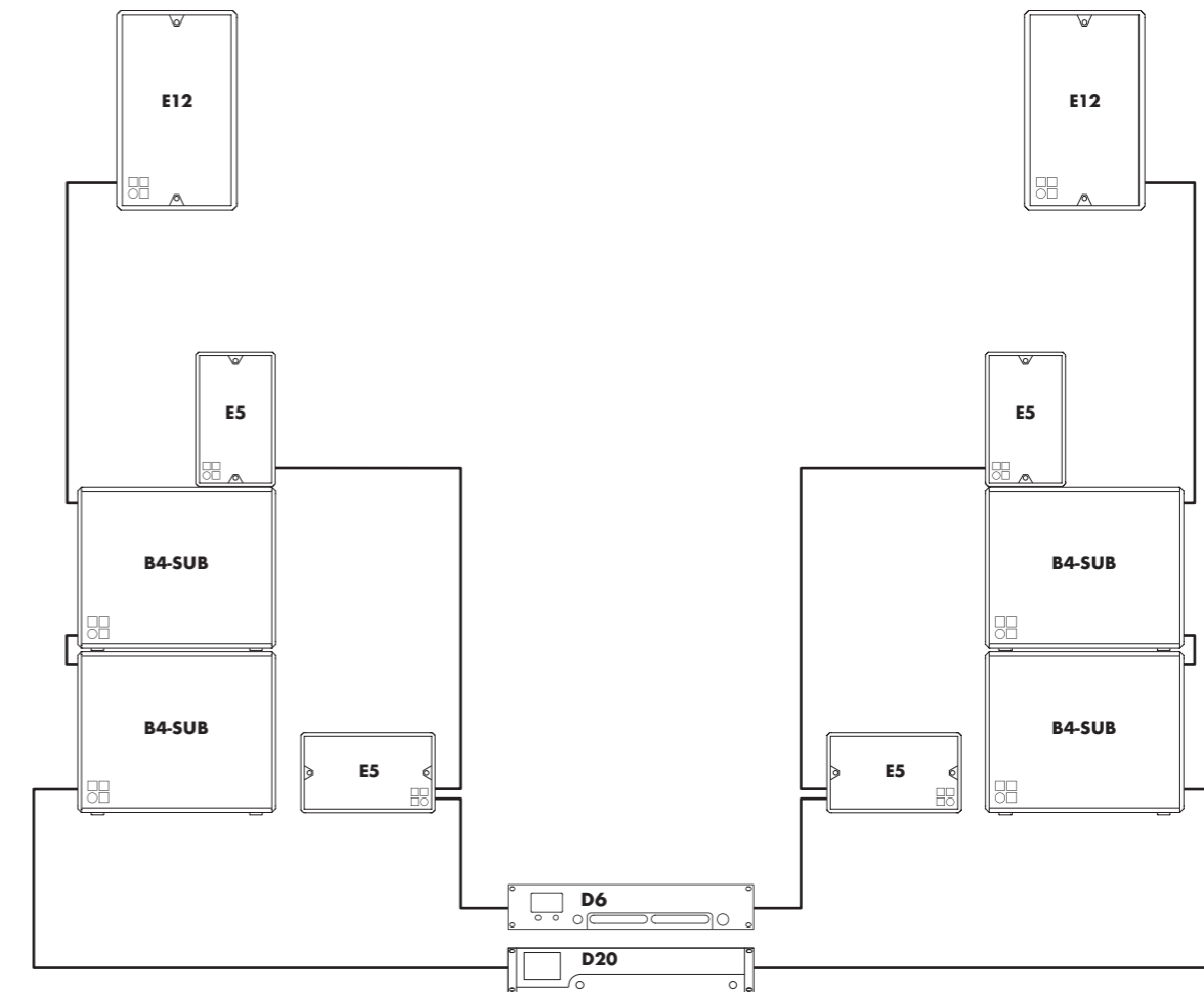
D20 amplifier in Mix TOP/SUB mode with E12 loudspeakers and B4 subwoofers as a powerful PA system and D6 amplifier in Dual Channel mode with E5 loudspeakers as nearfills
