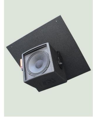
This new unit will be introduced at Barcelona CineEurope 2015. It is a 8" coaxial driver two way full range cinema surround speaker, designed with installation easiness for the new multichannel 3D sound systems in mind. With its directivity of 90°x90°, it can be installed at ceilings, as well as on standard on-wall applications.
