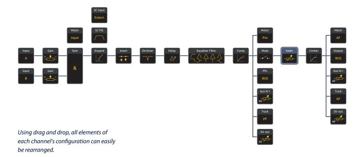
All in all, the DSP offers ten EQs or filters per channel: four full-parametric EQs, a high-shelving and a low-shelving filter, a high-pass and a low-pass filter, as well as two notch filters. The frequency settings of all EQs and filters are freely adjustable across the entire audio range from 20 Hz to 20 kHz.
