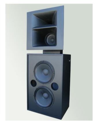
With the digital cinema in mind, we introduce this evolution of our LW 5007, a 3 way system for bi-amp with built-in network for mid-high. 2x15" bass loudspeakers + 1x10" midrange loudspeaker + 1,75" PM4 driver.
